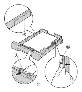
5 Insert the paper input tray to the unit, lifting the front part of the tray. Then push it completely into the unit.
